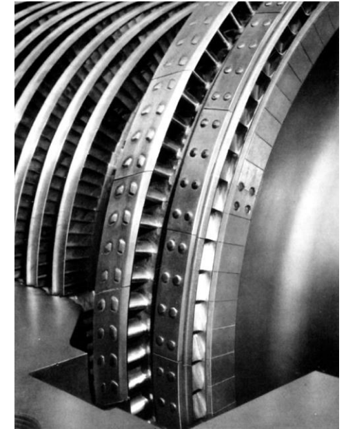
HP turbine Curtis stage
