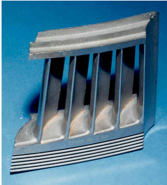
High temperature blades were made from forged bar with integral roots and shrouds, brazed into segments
