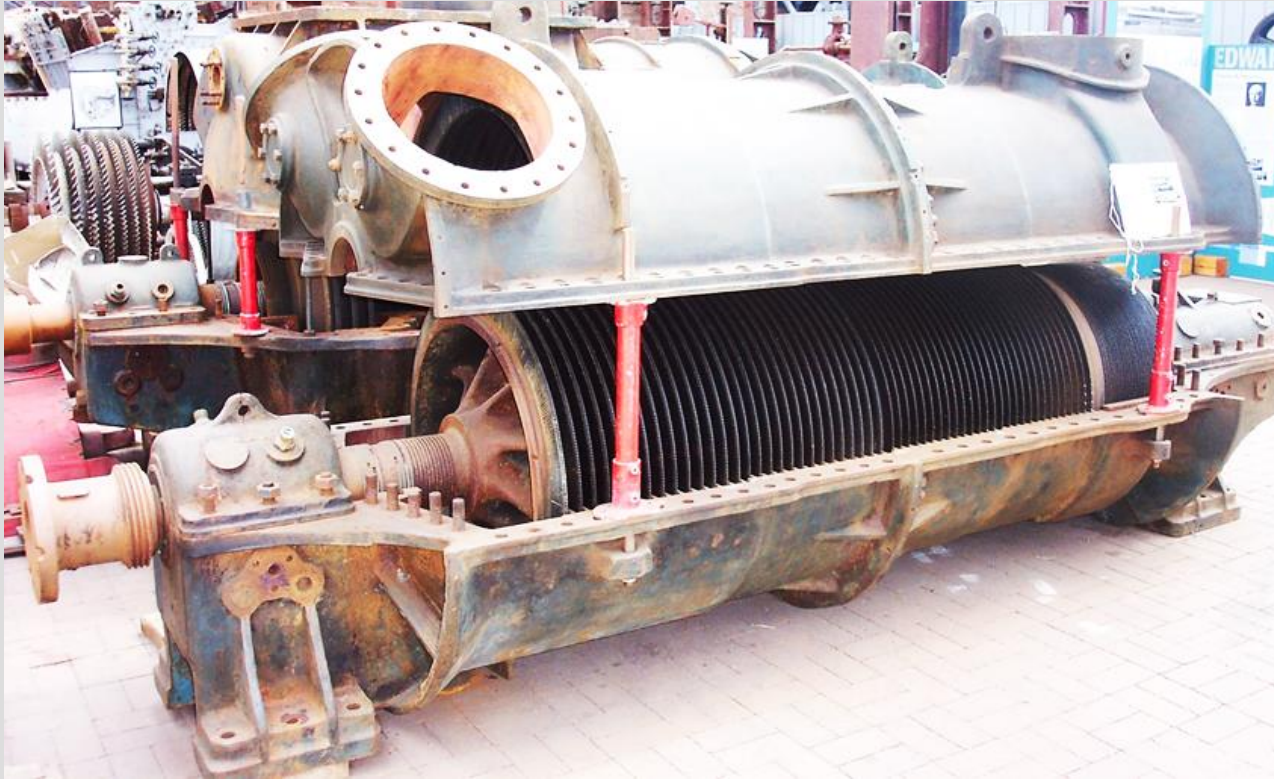
The high pressure turbine of TS King Edward
